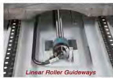
High precision linear roller guideways improve machining quality.
